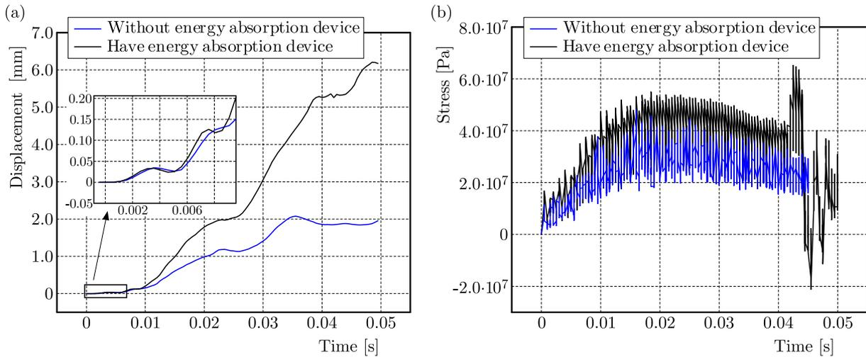
Fig. 9. Displacement/stress change curves of the same supporting system under different working conditions: (a) hydraulic cylinder, (b) position of the column top
