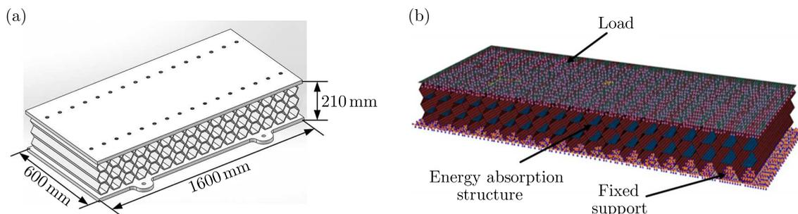
Fig. 5. Impact resistant structural model: (a) 3D-model, (b) FEM model
