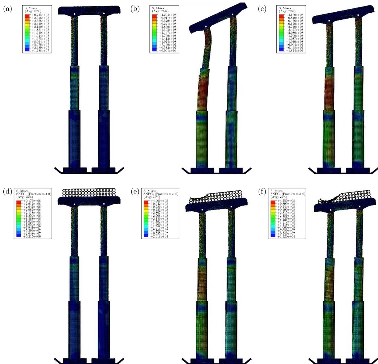
Fig. 10. Mechanical response of the hydraulic support under different impact loads: (a)-(c) without the energy absorption structure, (d)-(f) with the energy absorption structure
