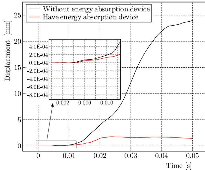
Fig. 11. Displacement curve of the hydraulic cylinder under a partial impact load
