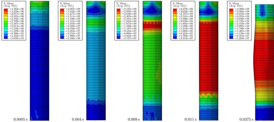
Fig. 8. Cloud diagram of hydraulic cylinder stress variation under the impact load
