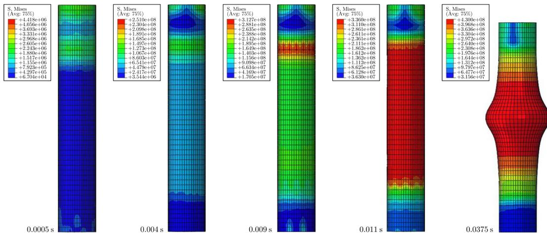
**Fig. 4.** Cloud diagram of hydraulic cylinder stress variation under the impact load
