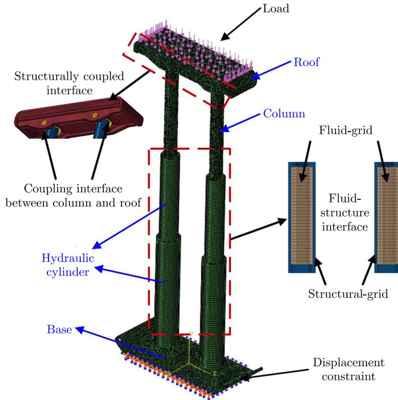
Fig. 2. Finite element model of the hydraulic support
