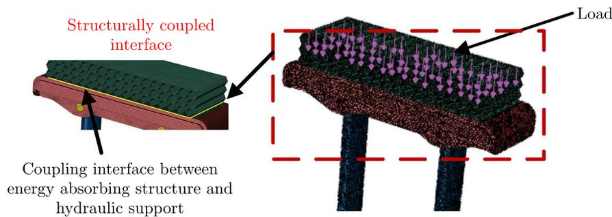
Fig. 7. Impact resistant hydraulic support model
