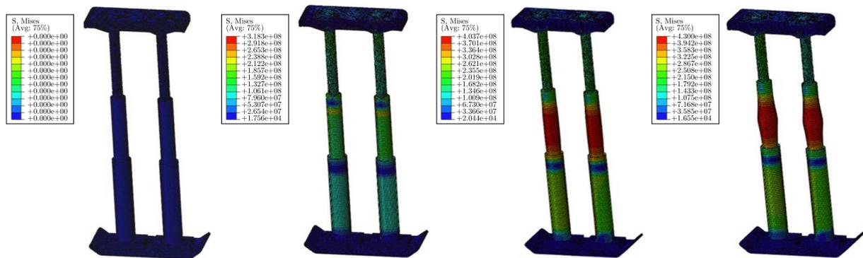
**Fig. 3.** Cloud diagram of the stress change of the hydraulic support machine
